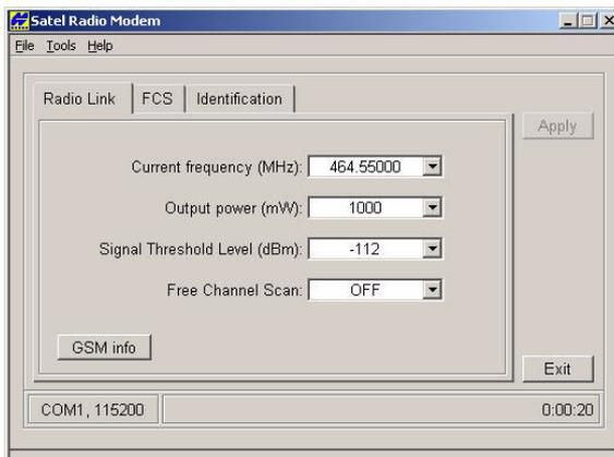
Figure 1-4. Radio Link Parameters Setup
