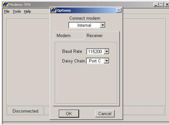
Figure 1-3. Modem-TPS Options for Receiver
