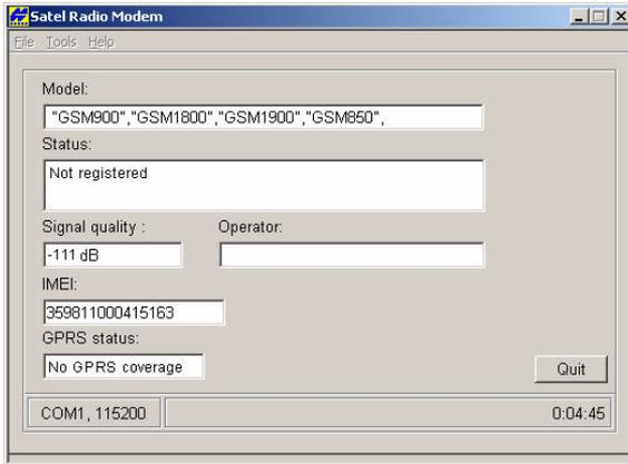
Figure 1-7. GSM Modem Parameters When Connection Fails
